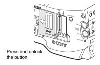
2 Press the EJECT button again to remove the card.
